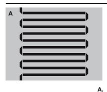
Spread the loose ribbon as shown in the figure, leaving the same distance between each string.
